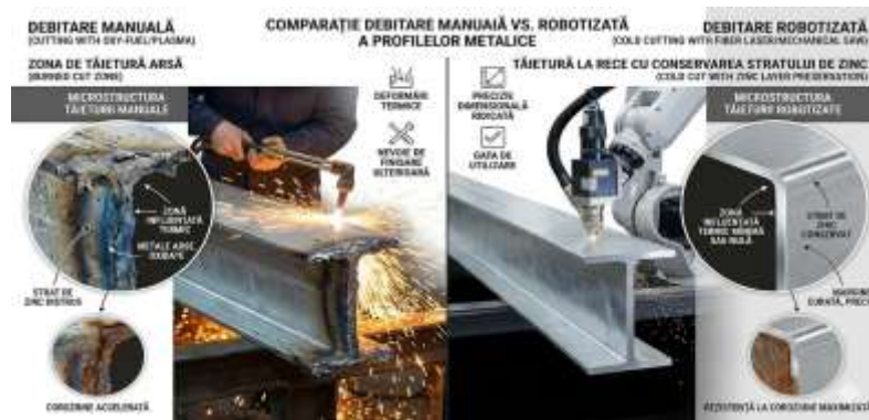
Fig. 1. Comparison of manual versus robotic cutting of metal profiles: the burned cut zone (left) — zinc burning at >419^{\circ}\text{C} with the angle grinder — versus cold cutting with preservation of the zinc layer (right), a robotic solution.
