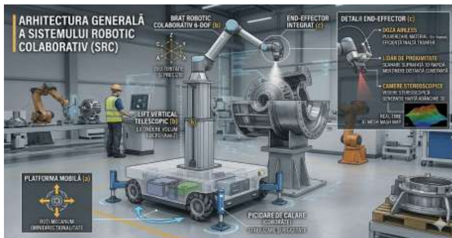
Fig. 2. General architecture of the Collaborative Robotic System (CRS): (a) the mobile platform with Mecanum wheels and levelling feet; (b) the 6-DOF arm with vertical lift; (c) the end-effector with Airless nozzle, proximity LiDAR, and stereoscopic cameras.
